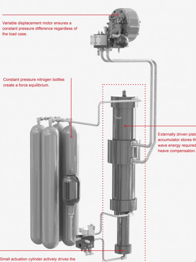
Small actuation cylinder actively drives the system based on a modified signal from a motion reference unit.
